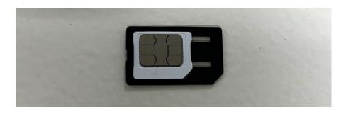
3) Remove the battery from the Wi-Fi device and insert the SIM card in the SIM card slot. The SIM card can only fit one slot in one direction:
